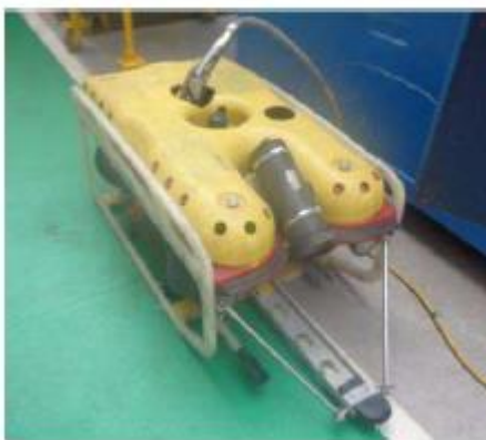
Figure 10: mini-ROV model Seaeye Falcon 12249 specs (for Pull-in and Pull-out operations)
